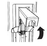
Open the station's door and pull out the connector.
