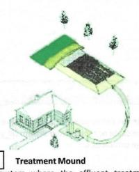
A system where the effluent treatment area includes a bed of sand and is built above ground to overcome limits imposed by proximity to water table or bed rock, or by highly permeable or impermeable soils.
