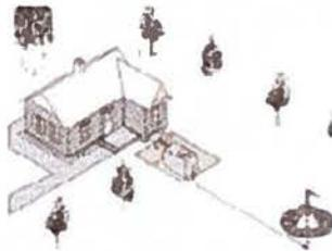
**Open Discharge (Pump Out) System**
