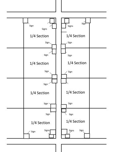
Sign to be placed at 45° angle facing traffic and situated on the sign post at a height of 3' to 6' from the ground. NO
