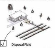
A system of treatment and disposal that distributes effluent within trenches containing void spaces that are covered with soil.
