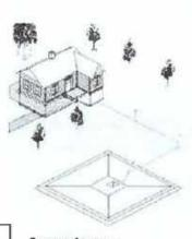
Sewage Lagoon A shallow artificial pond for the stabilization of sewage or effluent.
