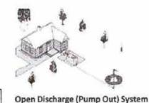
A system designed to discharge effluent to the ground surface to accomplish evaporation and absorption of the effluent into the soil.
