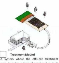
area includes a bed of sand and is built above ground to overcome limits imposed by proximity to water table or bed rock, or by highly permeable or impermeable soils.
