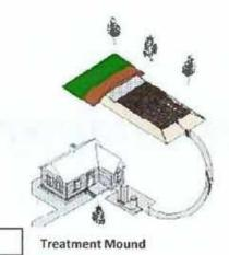
A system where the effluent treatment area includes a bed of sand and is built above ground to overcome limits imposed by proximity to water table or bed rock, or by highly permeable or impermeable soils.
