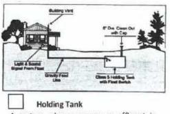
A system where sewage or effluent is retained in a tank until it can be transferred into mobile equipment for disposal elsewhere.
